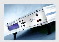
Can be directly connected to the magnetizing fixture for measurement of the total flux of the rotor where the measuring is provided.
